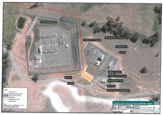
Figure 2: Existing substation and proposed substation expansion (Figure 2.4 in the statement of environmental effects accompanying development application 122/2017).
